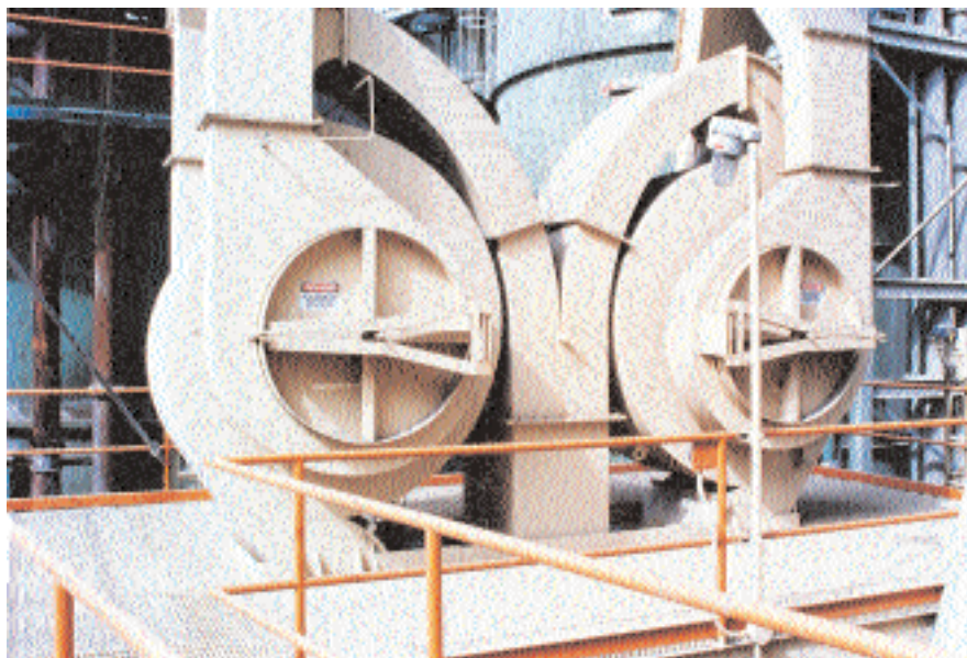
Each centrifugal classifier at the Four Corners Power Plant processes fly ash at a 40-t/h capacity.
